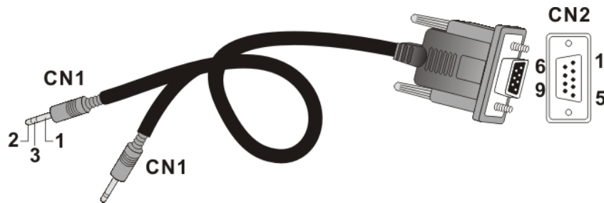
Figure C-3: COM1 Cable CN1 and CN2 Connectors
